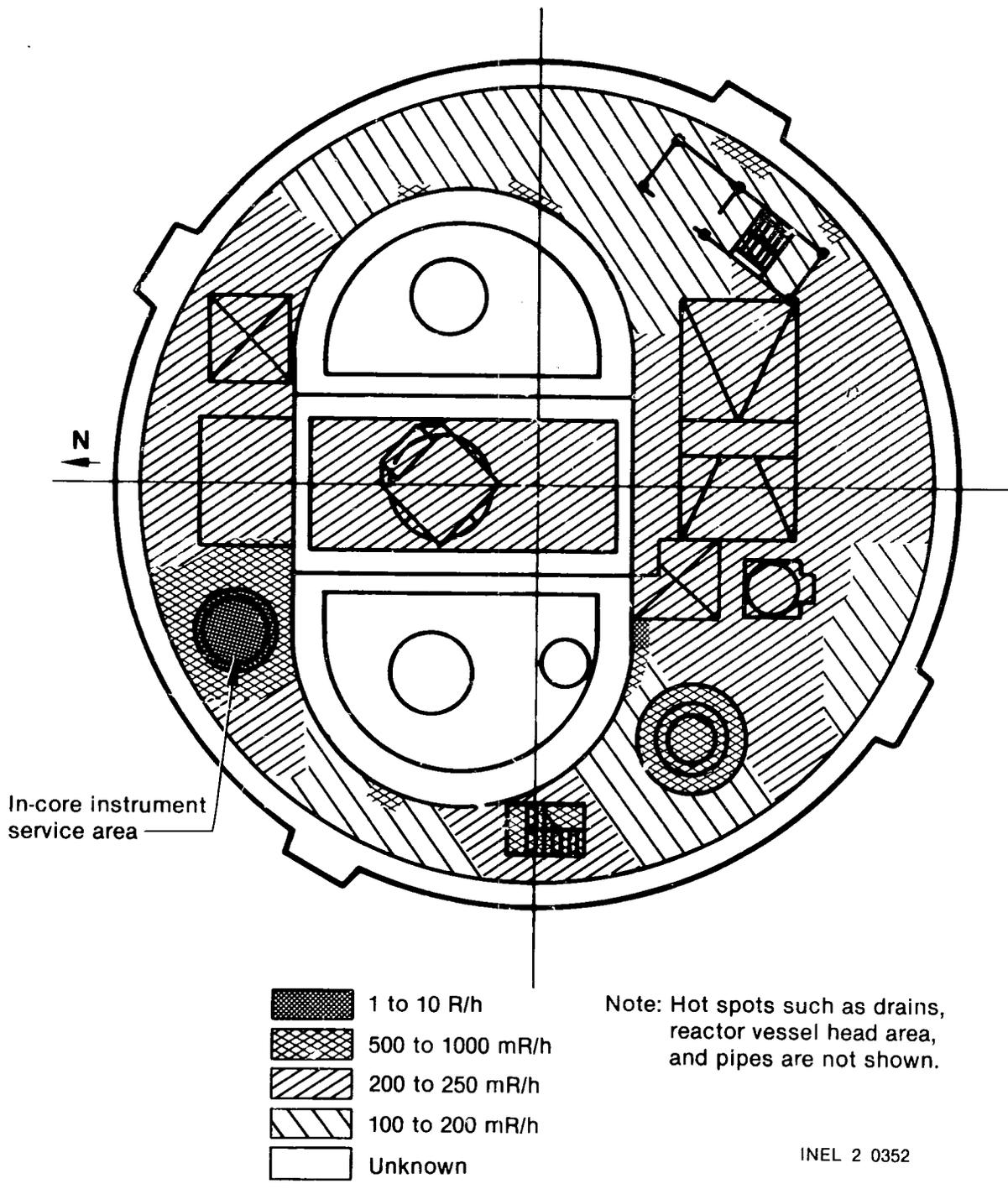
Figure 13. General radiation levels on 347-ft elevation.
