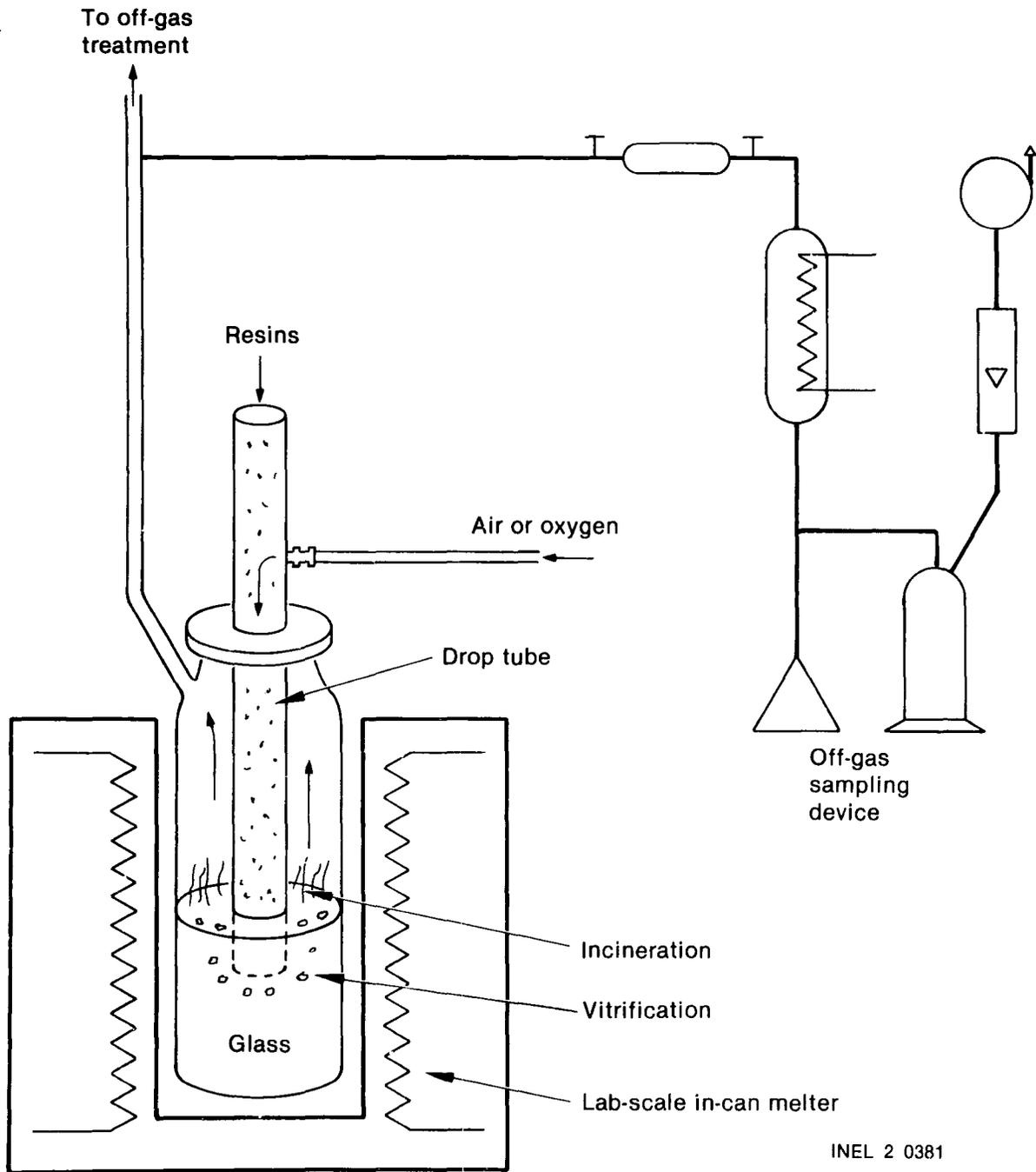
Figure 43. Laboratory-scale organic vitrification system.
