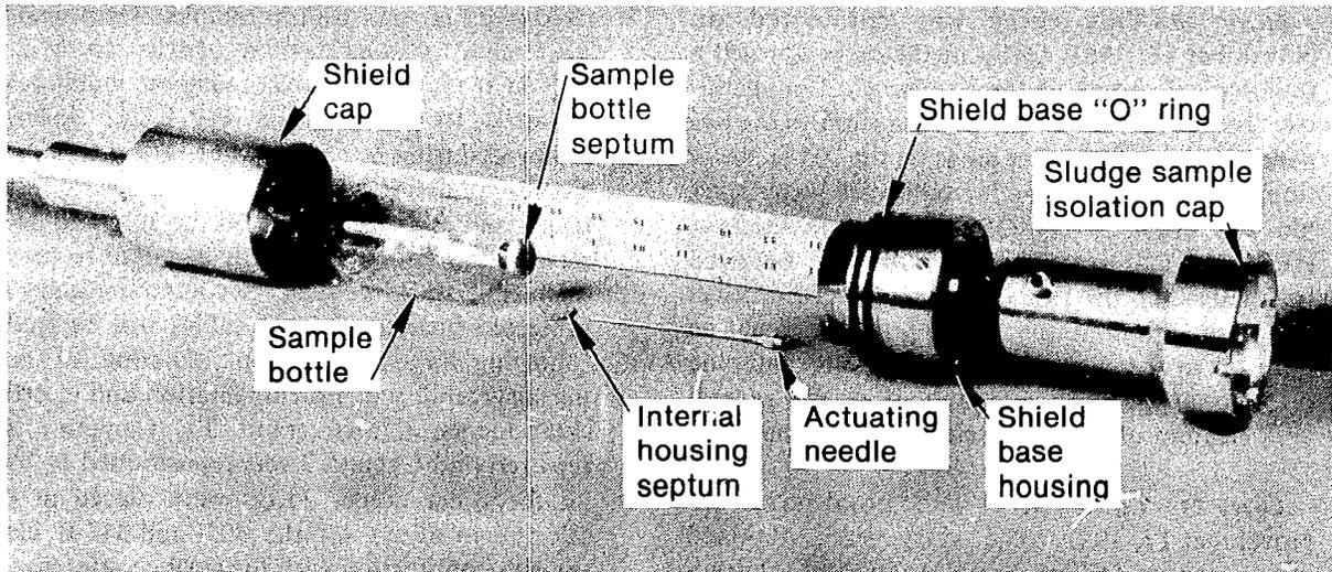
Figure 32. Single-level sump sampling device.
