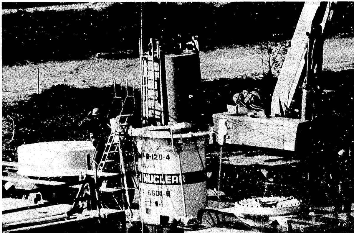
Figure 34. EPICOR II PF-16 liner loaded for shipping.
