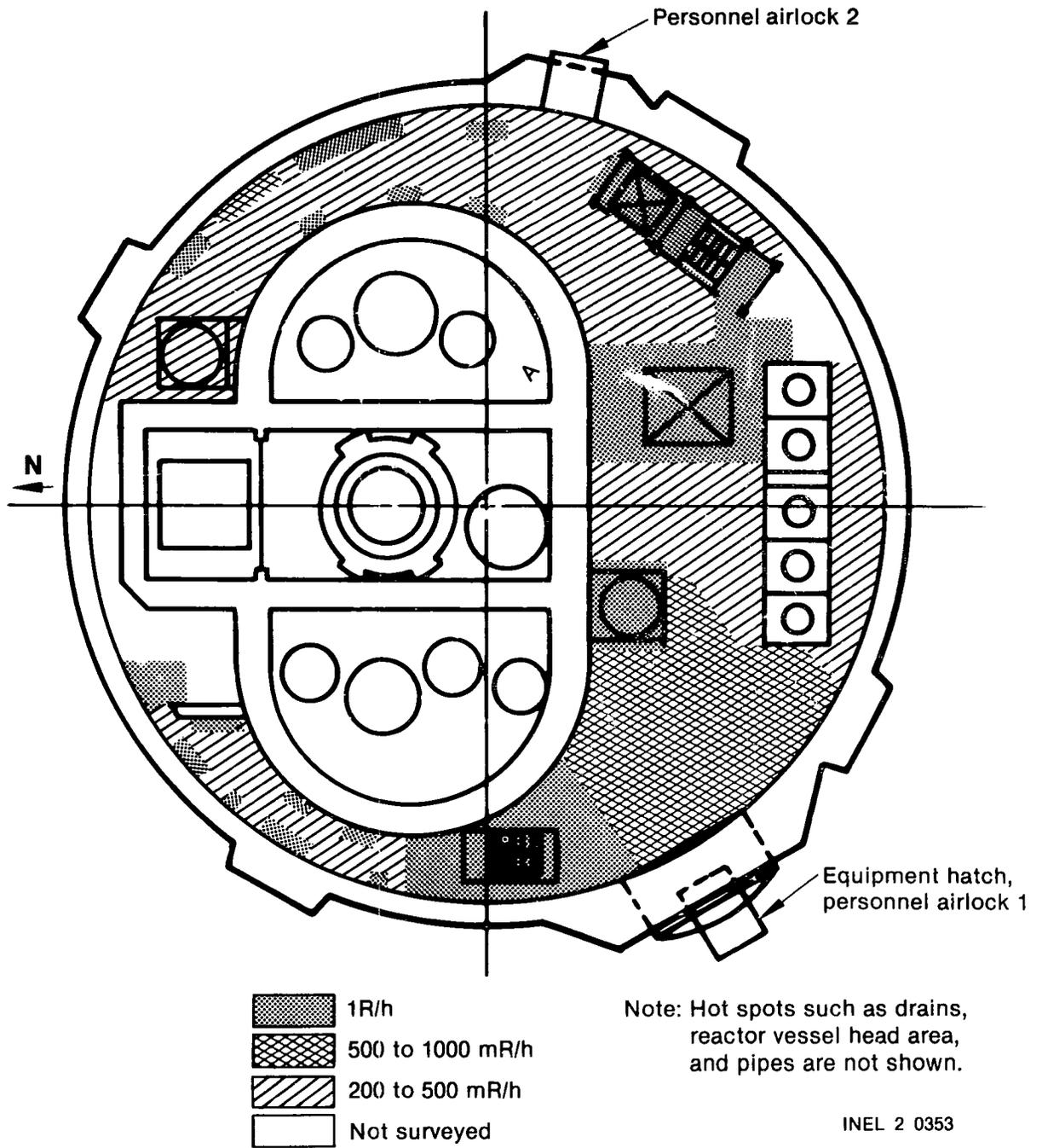
Figure 12. General radiation levels on 305-ft elevation.
