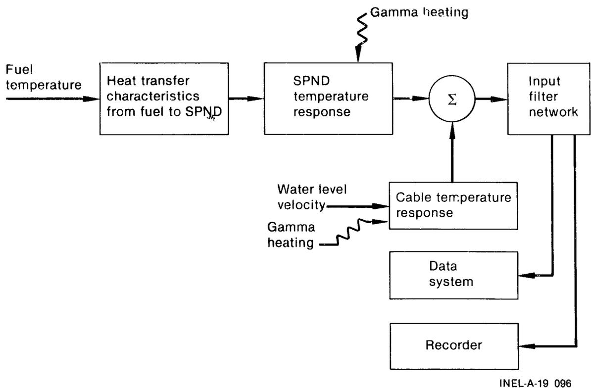
Figure 9. SPND measurement system block diagram.
