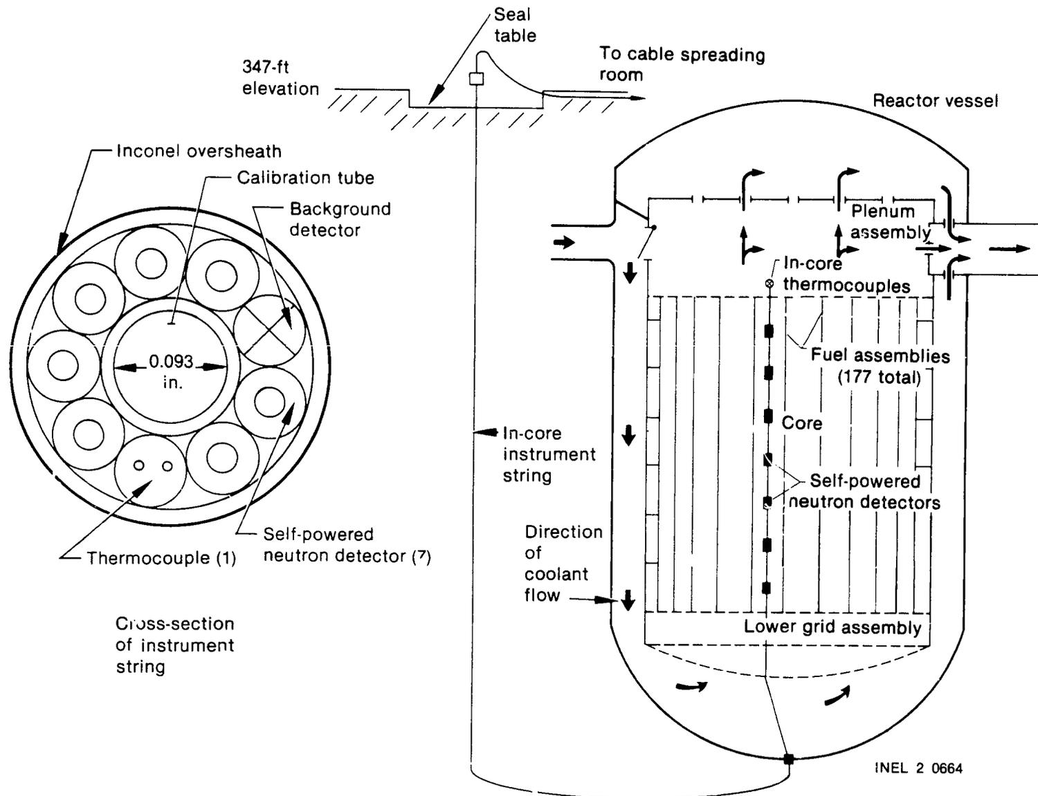
Figure 46. In-core instrumentation string orientation.
