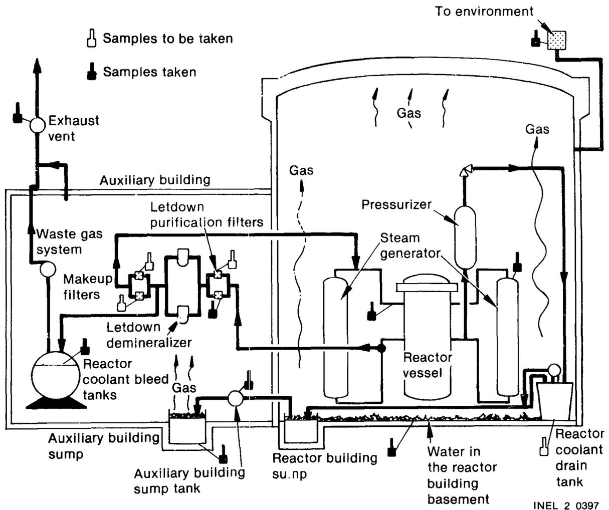
Figure 11. Reactor and auxiliary building sample points.
