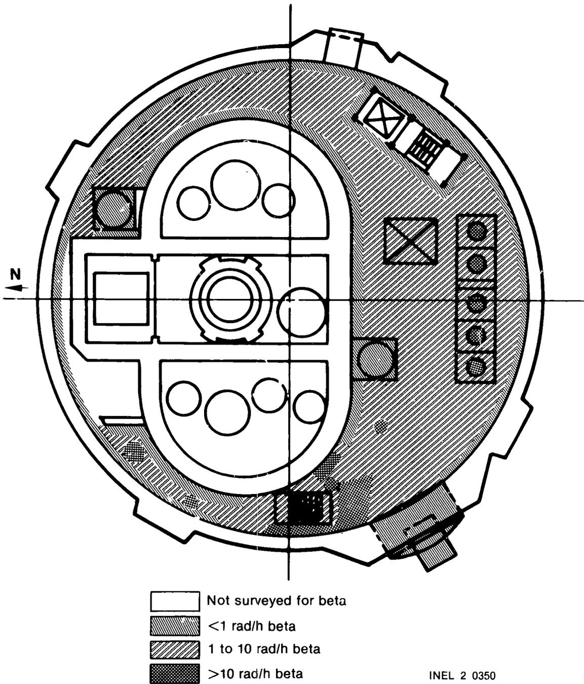
Figure 14. Beta radiation levels on 305-ft elevation.
