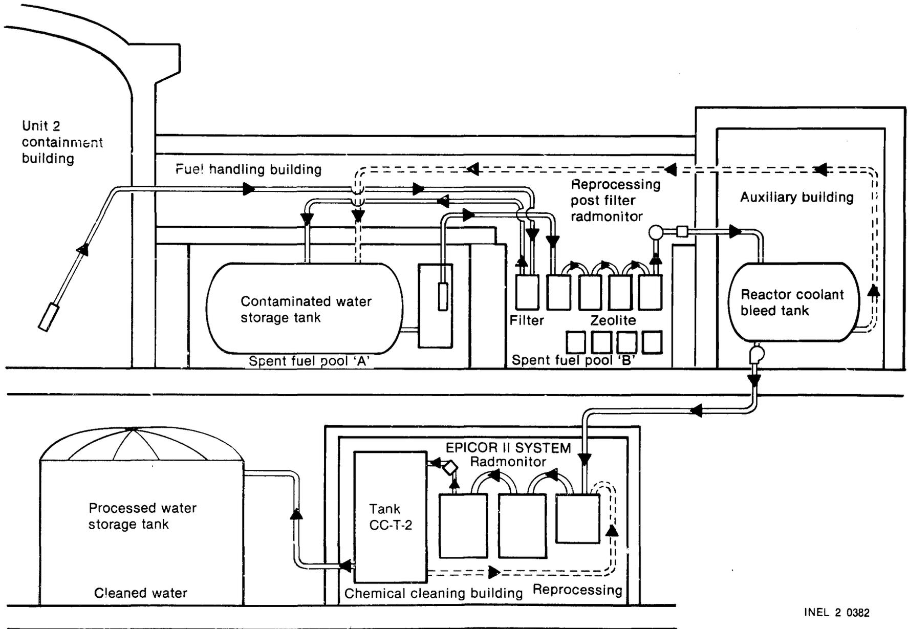
Figure 38. TMI-2 Submerged Demineralizer System.
