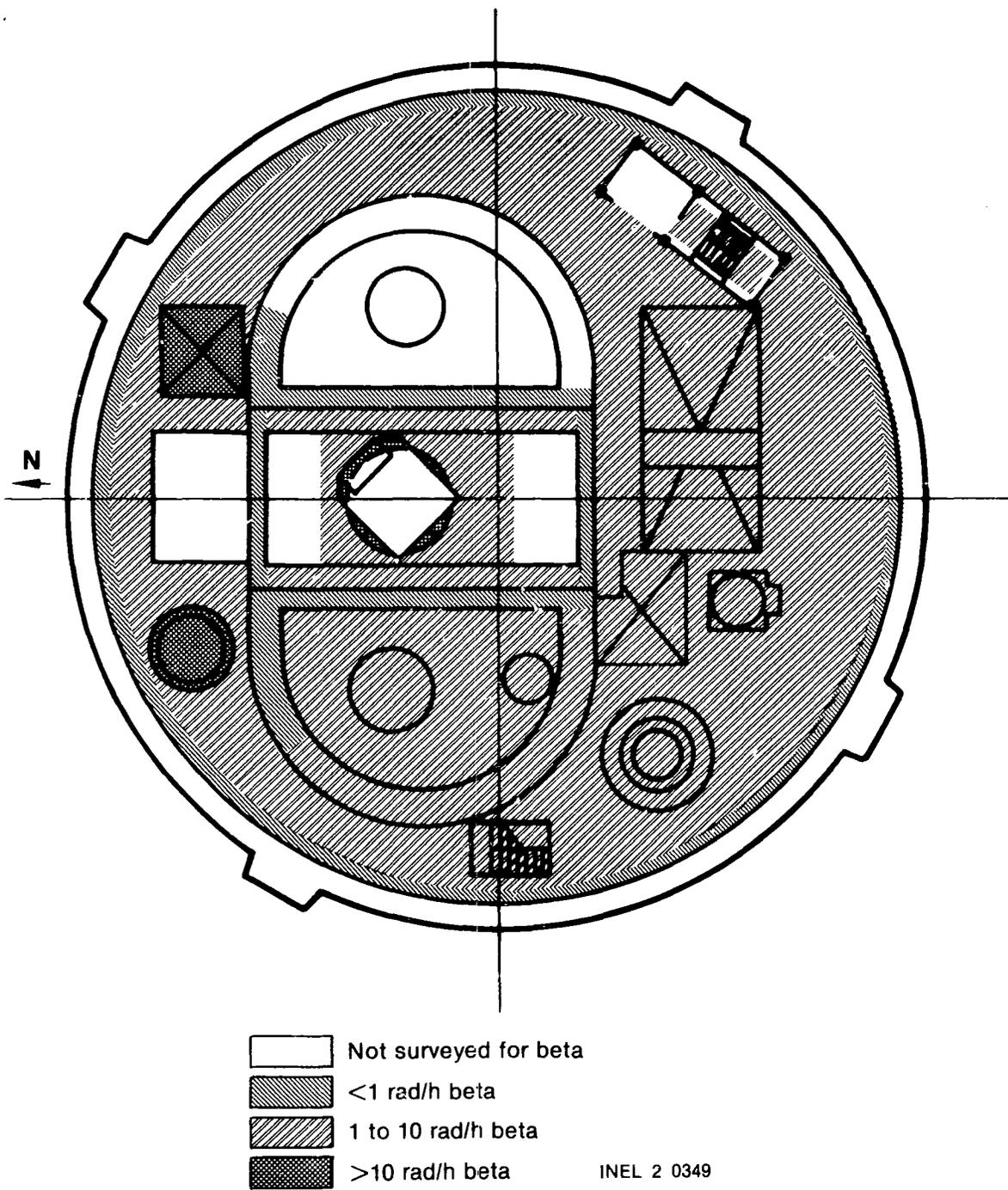
Figure 15. Beta radiation levels on 347-ft elevation.
