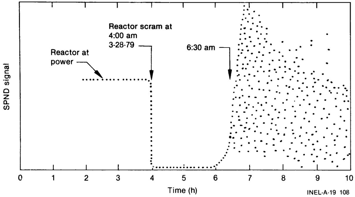
Figure 8. Backup recorder's tracing of in-core detector signals.
