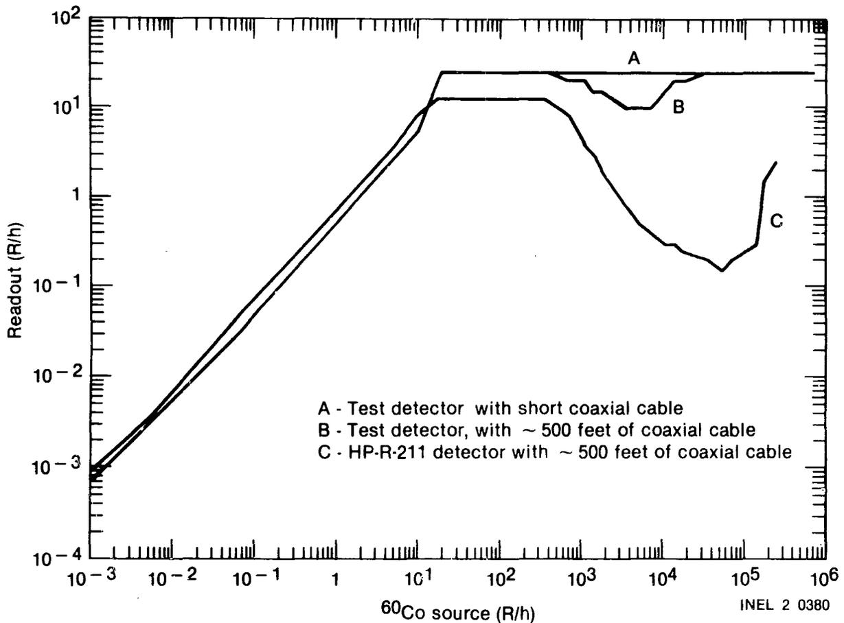
Figure 5. HP-R-211 multivalued readout.
